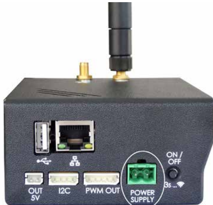
Figure 2-15 – Connection of the 2-pin connector to the 8-30 VDC IQ-LINK input
