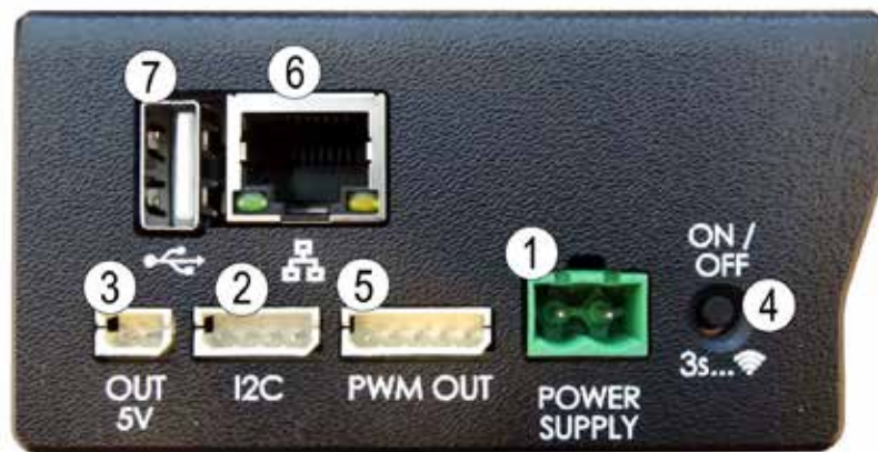
Figure 1-5 – IQ-LINK top panel connections
