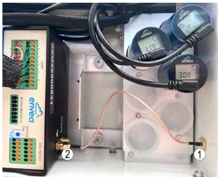
Figure 2–3 – Connection of antenna cable to IQ-LINK
