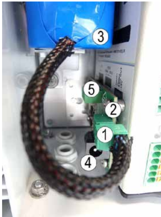
Figure 2–13 – Battery connection to the power supply board
