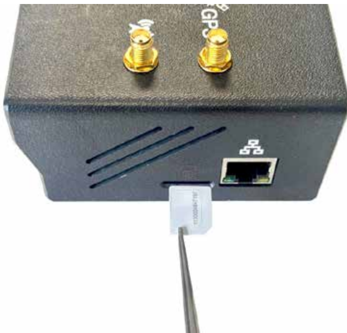
Insertion direction of the Anti mistake index
