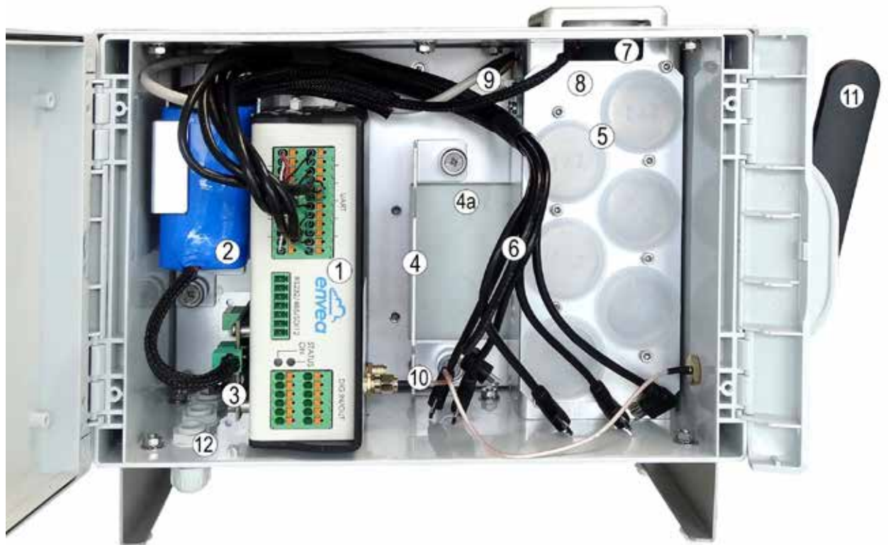
(1) IQ-LINK electronic box (1), (2) battery, (3) BQM board, (4) angle-bracket, (4.a) CAIRSENS PM location, (5) plugs to close the gas CAIRSENS location, (6) micro-USB cables, (7) fan, (8) manifold, (9) temperature probe, (10) coaxial cable for connecting the IQ-LINK to the external antenna, (11) radio antenna, (12) cable glands.
