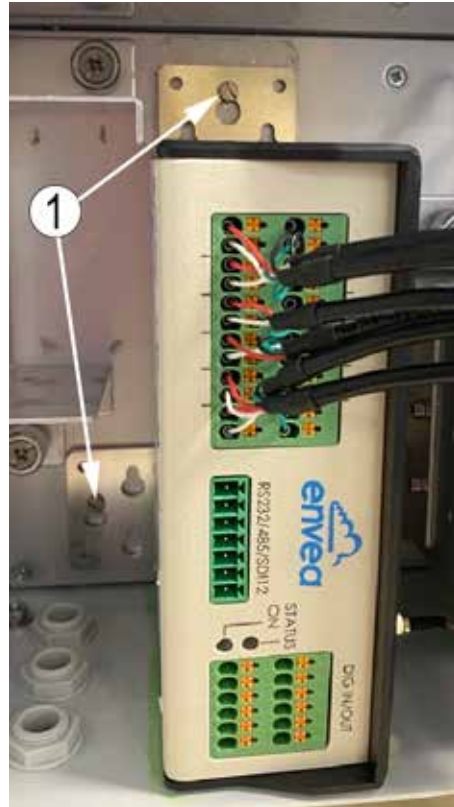
Figure 2–4 – Screws of the brackets holding the IQ-LINK
