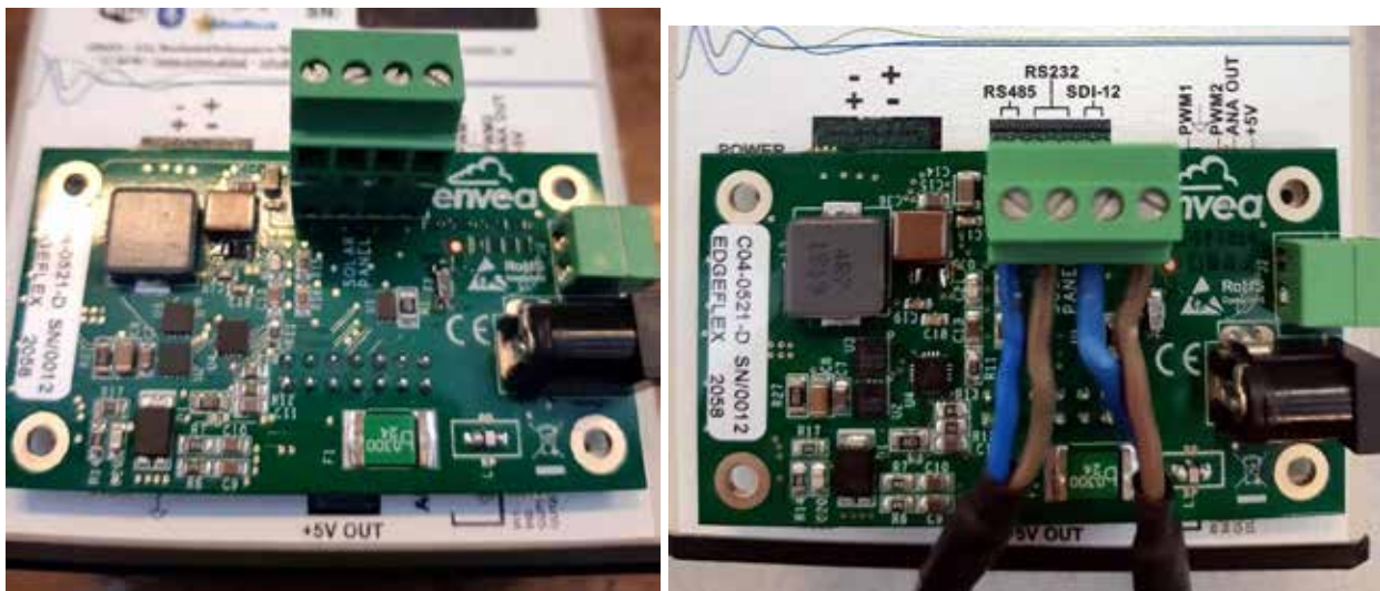
Figure 2–18 – Solar panel wiring on the power supply board
