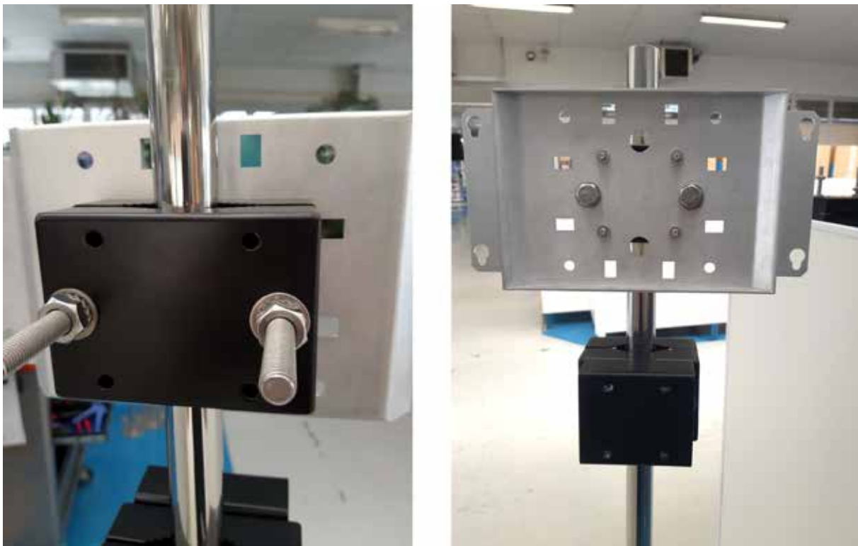
Figure 2–16 – Fixation of CAIRNET holder and solar panels on the tripod mast
